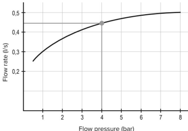
Example: Flow pressure 4 bar  $\Rightarrow$  Flow rate 0.44 l/s  $\Rightarrow$  with 5 s flush time  $\triangleq$  2.2 l flush volume
