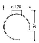
Abmessungen in mm
